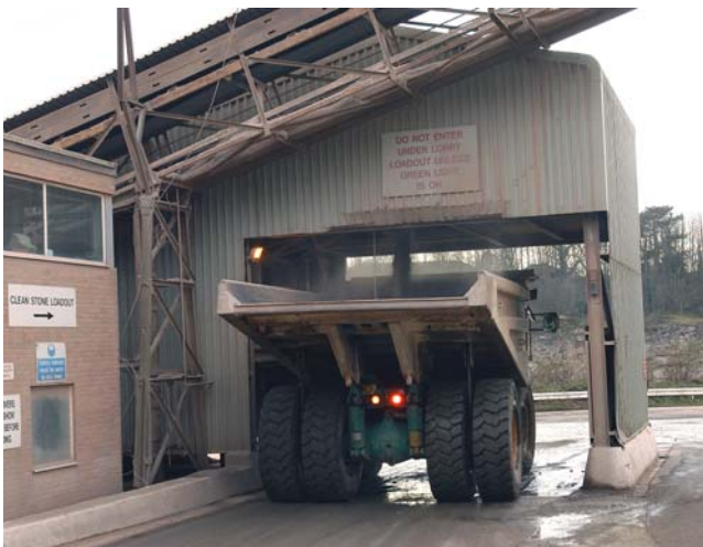
5. Loading dumper with finished aggregate
