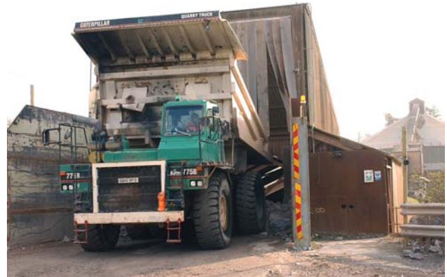
4. Tipping rock into crusher
